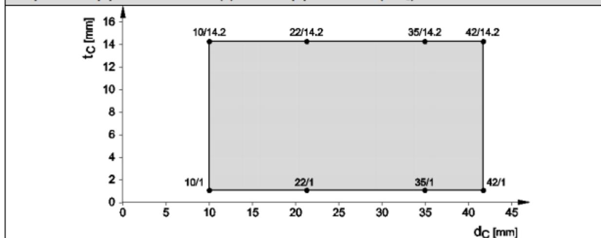
Copper pipes, wall ( $\geq 100$  mm) – EI 90, C/U (plus AP1 or AP3)
