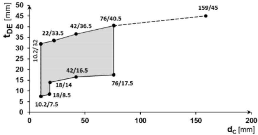
**Steel pipes, wall ( $\geq 100$  mm) – EI 90, C/U plus AP1**
