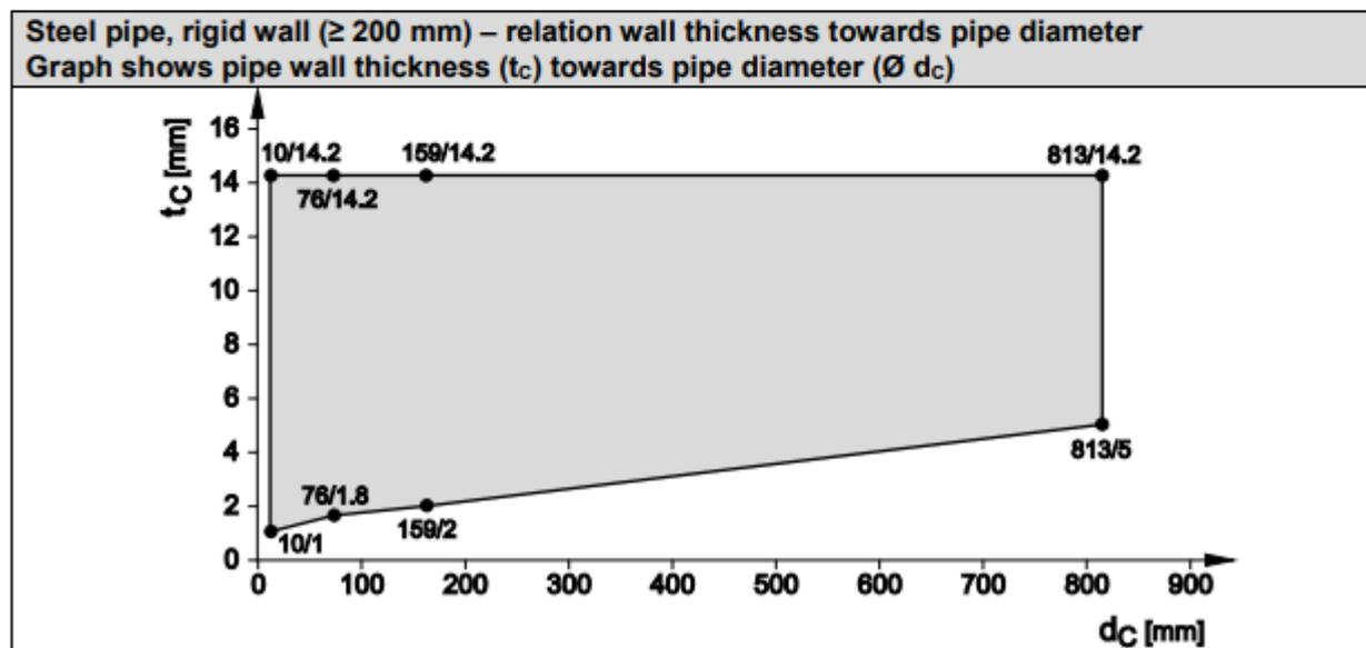
Steel pipes, C/U, rigid wall ( $\geq 200$  mm) – EI 120 /90, C/U
