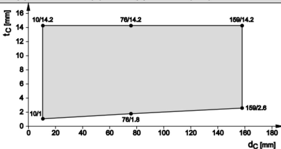
**Steel pipes, flexible wall ( $\geq 100$  mm) – EI 90 / EI 120 (dotted line) C/U**
