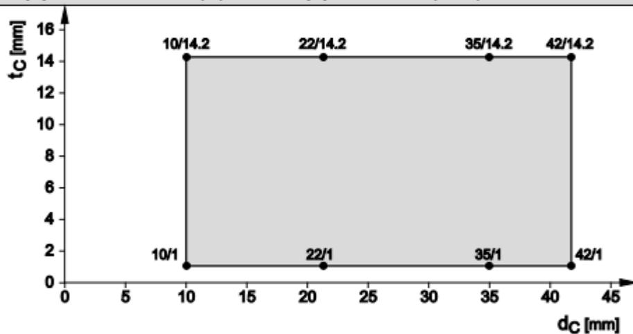
**Copper pipes, rigid wall ( $\geq 200$  mm) – EI 120 / EI 90, C/U
