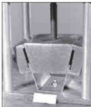
Pull-over test specimen at test start
